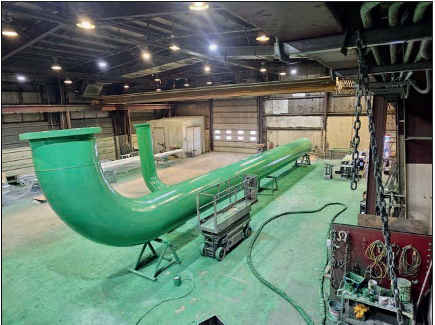
Complex designs made maneuvering, handling and coating such large spools a challenge.
