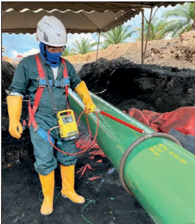
Below & right: Holiday testing of the cured Protal 7200.
