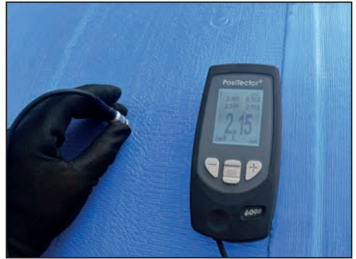
Above: Testing the coating thickness.
