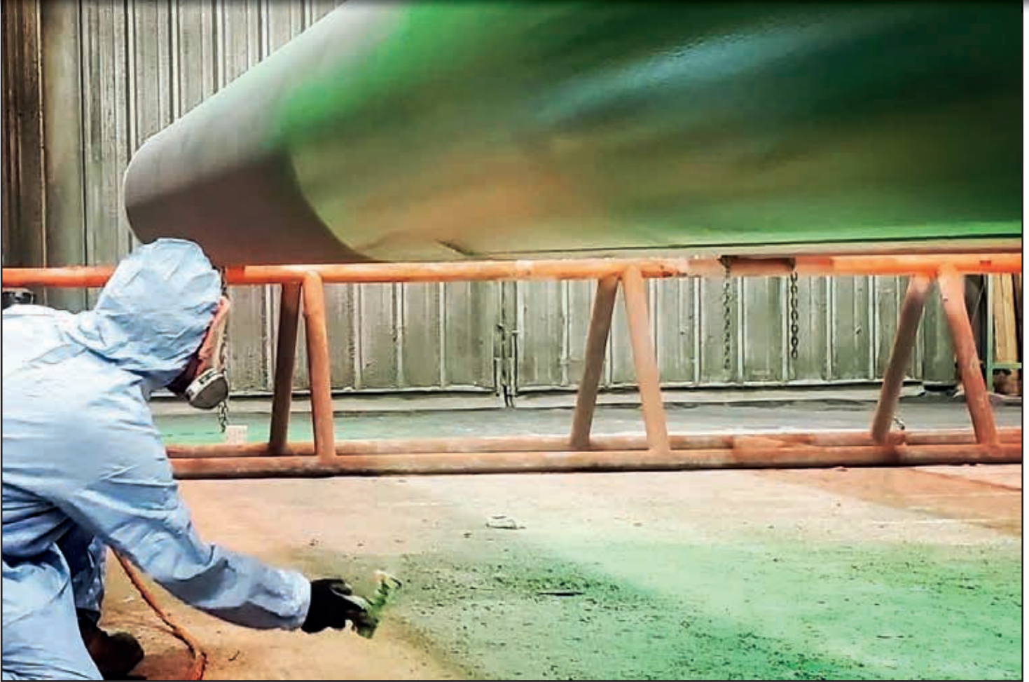
Above: Plural Spray Application of Protal 7200.
