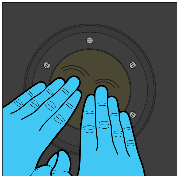
Fig. 3: Flatten the mastic, avoiding the threaded areas.
