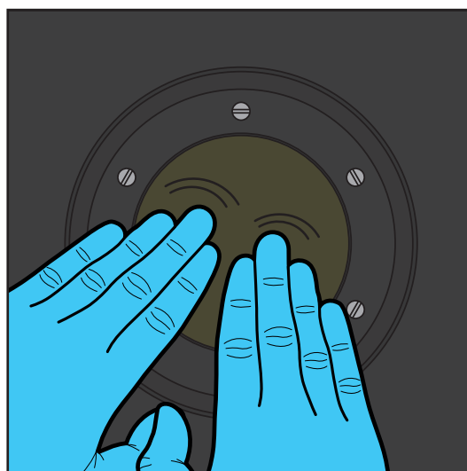
Fig. 8: Return the mastic to the inspection port and flatten.
