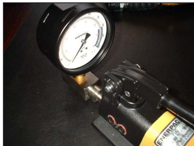
Fig. 3: The gauge and gauge adaptor in place.
