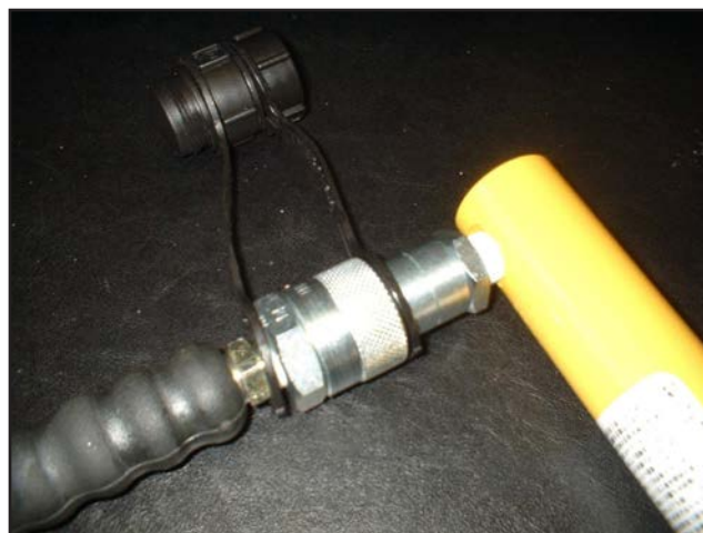
Fig. 6: An assembled coupling. Note the stowage of the dust caps.
