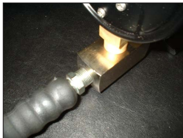
Fig. 4: The hose connected to the gauge adaptor.
