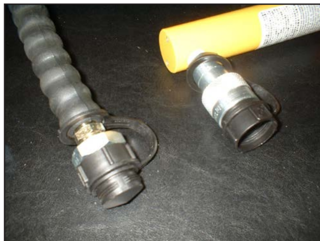
Fig. 5: The dust caps in position.
