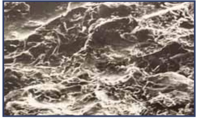
500 x magnification of a steel plate wet-abrasive blasted with HoldTight 102
