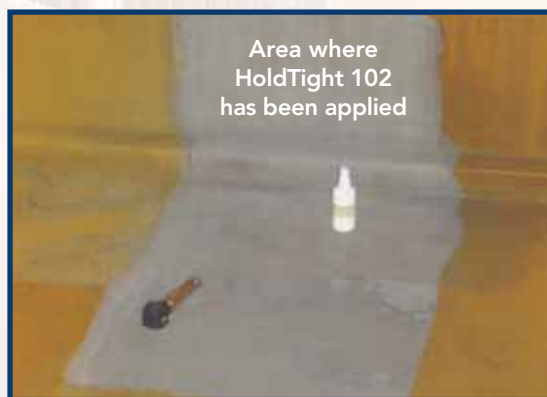
Above: View inside a tank where HoldTight 102 was applied to a panel. Note the flash rust that has appeared on the untreated area. The treated HoldTight 102 area will remain rust free for up to 48 hours or longer after application.
