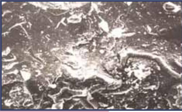
500 x magnification of a steel plate dry blasted
