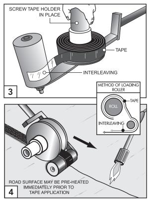
one turn to expose the bitumen compound (as Fig 2). Pass the tape around the application roller (as Fig 3). Push the roller along the line of the crack as shown (as Fig 4) to apply the tape centrally over the crack. Press the tape down thoroughly and remove the interleaving. Traffic may flow immediately.
