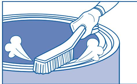
Fig 1. Joint surfaces should be sound, clean and dry before priming
