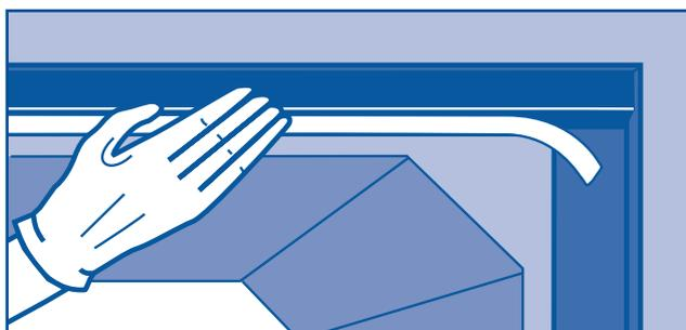
Fig 5. Densostrip is heated on one side and pressed firmly into position
