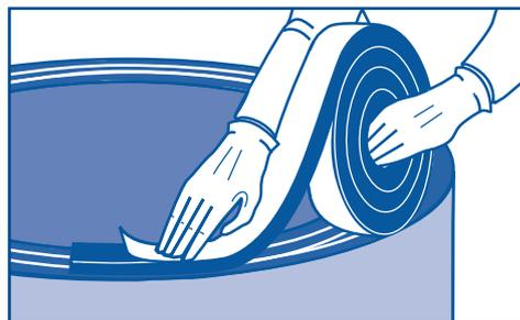
Fig 3. Apply Densostrip across the groove and remove the interleaving
